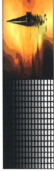
When the brightness of traditional outdoor LED display decreases to indoor use, the gray scale will be damaged seriously, and not able to show image details.
